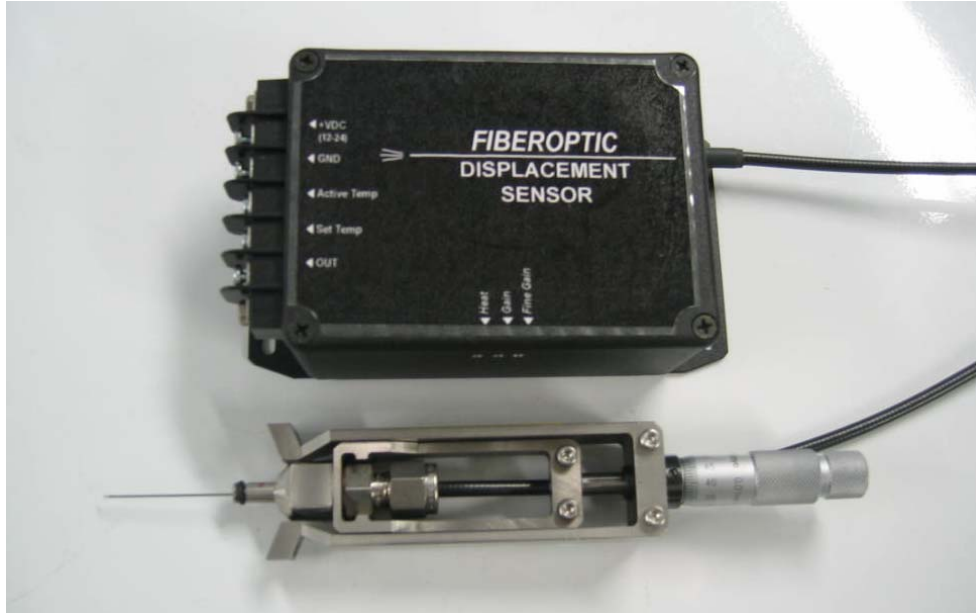
Figure 5-12: Laser Displacement Sensor ( \phi 0.8mm ) used for Speed Measurement.
