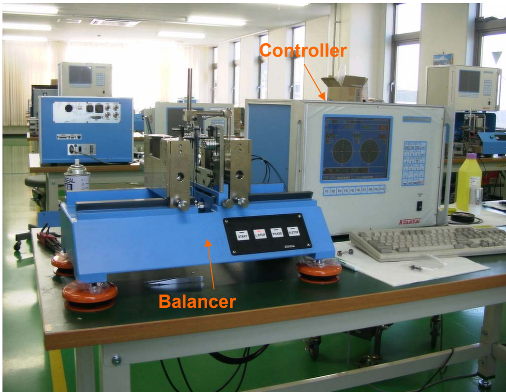
Figure 4-26: The Micro-Balancer Developed for Micro-High-Speed Rotor.
